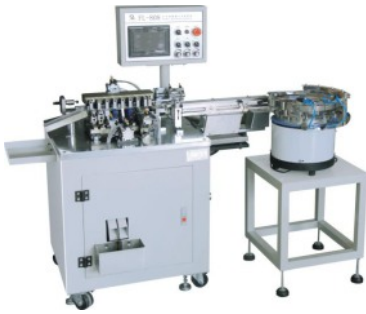
PREFORMING RADIAL COMPONENTS
