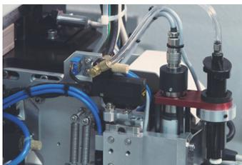
With pin-in-paste technology, through-hole (PTH) component placement can follow the SMD component placement process, with both being reflowed together in the oven. Using our solder paste dispenser, plated-through component holes are filled before the insertion of the components. This eliminates the wave soldering process altogether to dramatically improve line throughput and efficiency.
