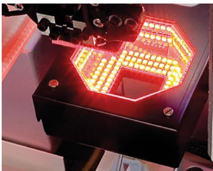
This high-resolution camera is used for inspection of ultra fine pitch components,  $\mu$ BGA, and flip chip devices. It's also used for components larger than the 50 mm x 50mm specification of the "on the fly" camera, to give accurate machine vision up to 99mm x 99mm.
