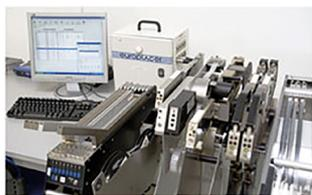
Set-up help facilitates the new product introduction from a programming station by preparing the machine loading for the next job without interrupting production.
