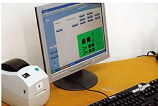
Offline programming stations can be set up on a standard PC hosting the Europlacer software suite.
