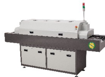
REFLOW OVEN WITH 3 HEATING ZONES
