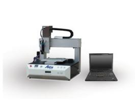
Every high-speed dispenser can provide various dispensing patterns. For example, single dots can be set to different sizes, based on what is required. The speed can also be adjusted – different speeds will create different line thickness. The flying pattern also ensures that there is fixed volume dispensed so as to minimize wastage, based on the length of dispensing that is adjusted according to the dispensing speed.
