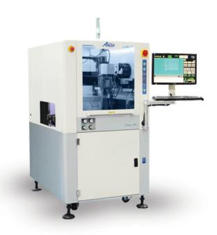
X3 is designed to strike a balance between cost and performance. Machine come with a single head 2 nozzles structure (spray and dispense) with 3 servo motors driven axis movement (X, Y, Z) as standard.
